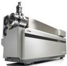
Liquid chromatography-tandem mass spectrometry (LC-MS/MS)
