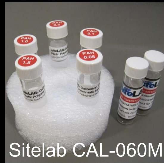
Sitelab CAL-060M PAH calibration kit used for analysis
