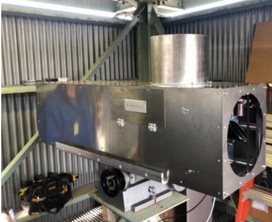
TDL Base Unit Installed on Mounting Platform
