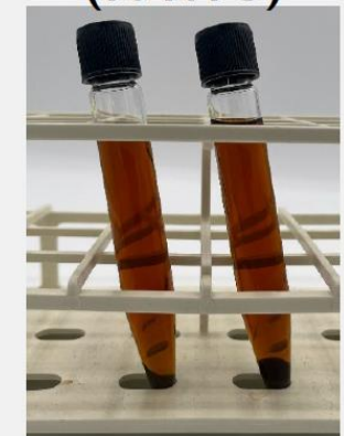
After 2800 RCF, 30 min Centrifuging (50 NTU)
