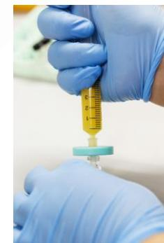
6. Filter through preconditioned 0.2µm PP syringe into 15mL centrifuge tube
