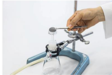
1 Place the filter using the supplied tweezers
