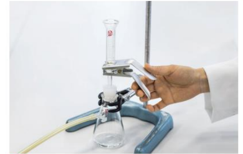
3 Secure the filtration assembly with the clamp
