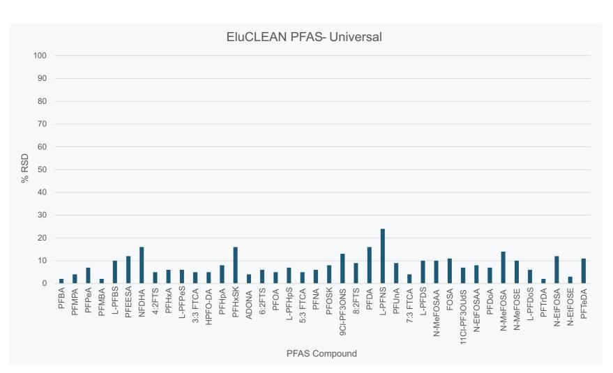
Figure 5: Results of Initial Demonstration of Precision (IDP) using the EluCLEAN PFAS – Universal cartridge.
