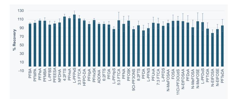
Figure 7: Results of Initial Demonstration of Accuracy (IDA) using the EluCLEAN PFAS – Universal cartridge.
