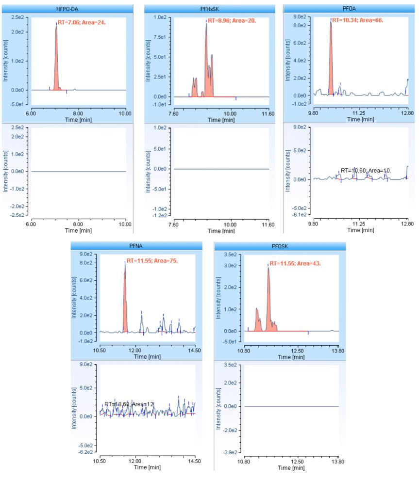
Figure 3: Overlay mass chromatogram comparisons of resulting of LOQ sample (upper) vs. blank sample (lower) processed using the FREESTYLE XANA-PFAS Tabletop robotic sampler for A). HFPO, B). PFHxS, C). PFOA, D). PFNA, and E). PFOS.
