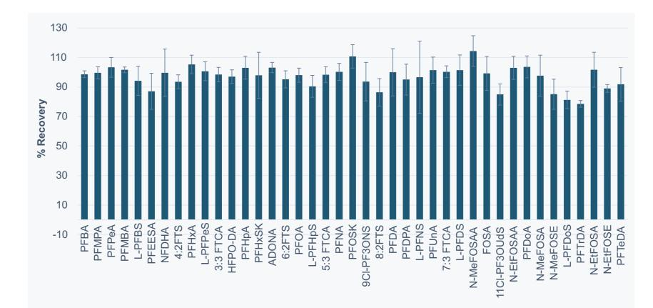
Figure 6: Results of Initial Demonstration of Accuracy (IDA) using the EluCLEAN PFAS – WAX/GCB cartridge.
