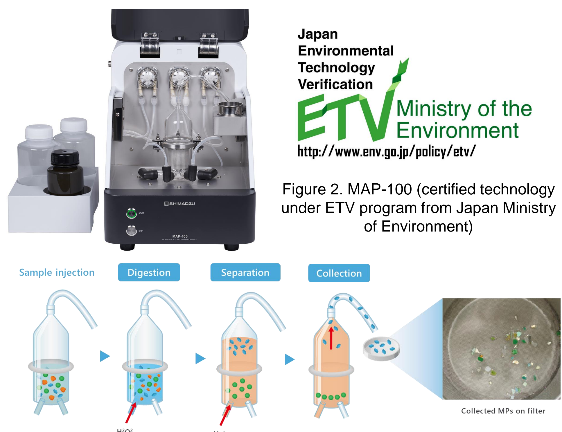
Figure 3. Sample preparation process using MAP-100
