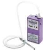
A Pumped sampling onto sorbent tubes
