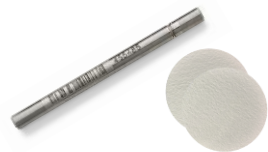
A Direct desorption of filters
