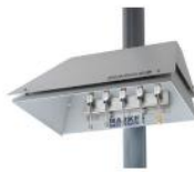
B Passive sampling onto sorbent tubes
