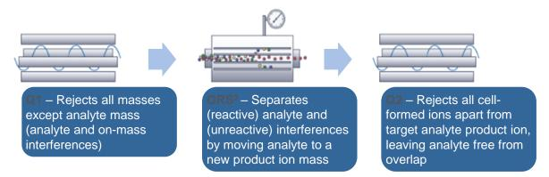
*ICP-QQQ MS/MS Mass Shift mode is simple and reliable, as Q1 rejects all non-target precursor ions, so the cell processes are consistent*
