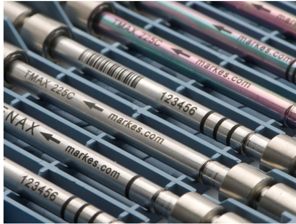
Automated sampling onto thermal desorption (TD) tubes containing PM2.5 filters instead of sorbent
