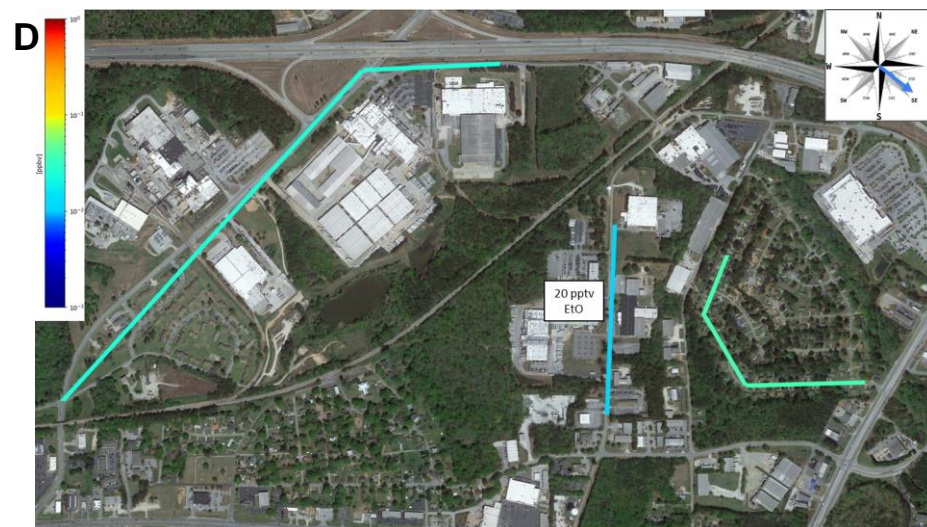
(D) EtO measurements at a sterilization facility in GA. Upwind and downwind measurements were made as well as at site, which is labeled by the boxes with EtO concentrations.
