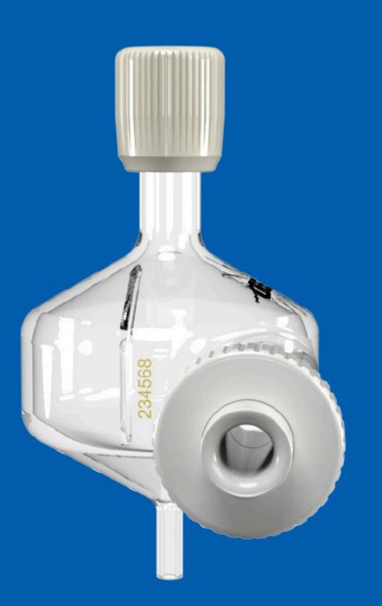
Within the IsoMist-MS Peltier is Glass Expansion's new Tracey™ DC spray chamber, a low-volume cyclonic design with Helix™ CT interface for superior analytical performance and washout efficiency.
