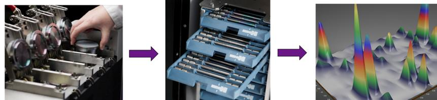
Tyre samples placed into a micro-chamber. Evolve compounds collected onto TD tubes
