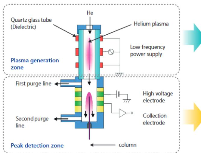
Three electrodes are placed on the quartz tube. High voltage is applied to electrodes, and plasma is generated
