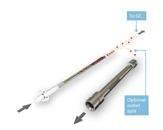
Focusing trap rapidly heated (up to 100°C/s) in a reverse flow of carrier gas ('backflush' operation)
