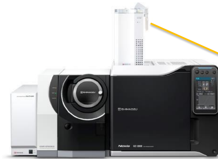
EGA/PY-3030D multi-shot pyrolyzer, AS-1020E auto-shot sampler (Frontier Laboratories Ltd.)
