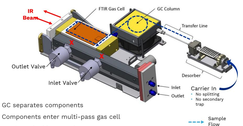
• Gas is probed by an IR beam
