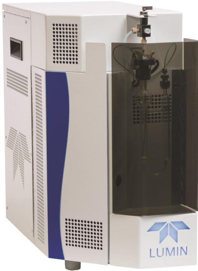
Utilizes Purge and Trap with excellent recoveries with most VOC. 1,4 dioxane is high water solubility with a very large partition coefficient thus the need for heated purge. The heated purge temperature significantly increases the water load on the trap/column thus lead to interferences by water.
