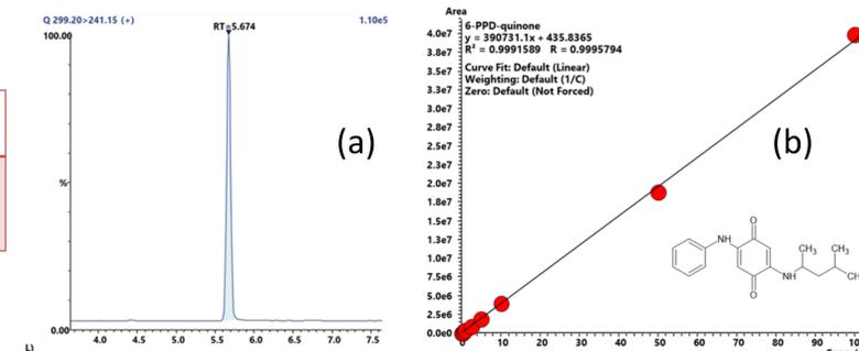
**Figure 2.** (a) Linear calibration curve for 6-PPD-quinone in the 0.01-100 ng/mL range. Inset: Chemical structure of 6-PPD-quinone. (b) Example MRM chromatogram for 6-PPD-quinone (m/z 299.20 > 241.15). Concentration of neat standard is 1 ng/mL.
