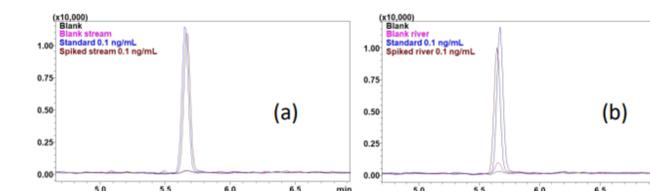
**Figure 5.** MRM overlay in (a) blank, standard, unspiked and spiked stream samples, (b) blank, standard, unspiked and spiked river samples.
