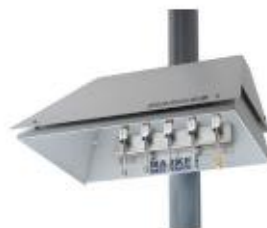
B Passive sampling onto sorbent tubes
