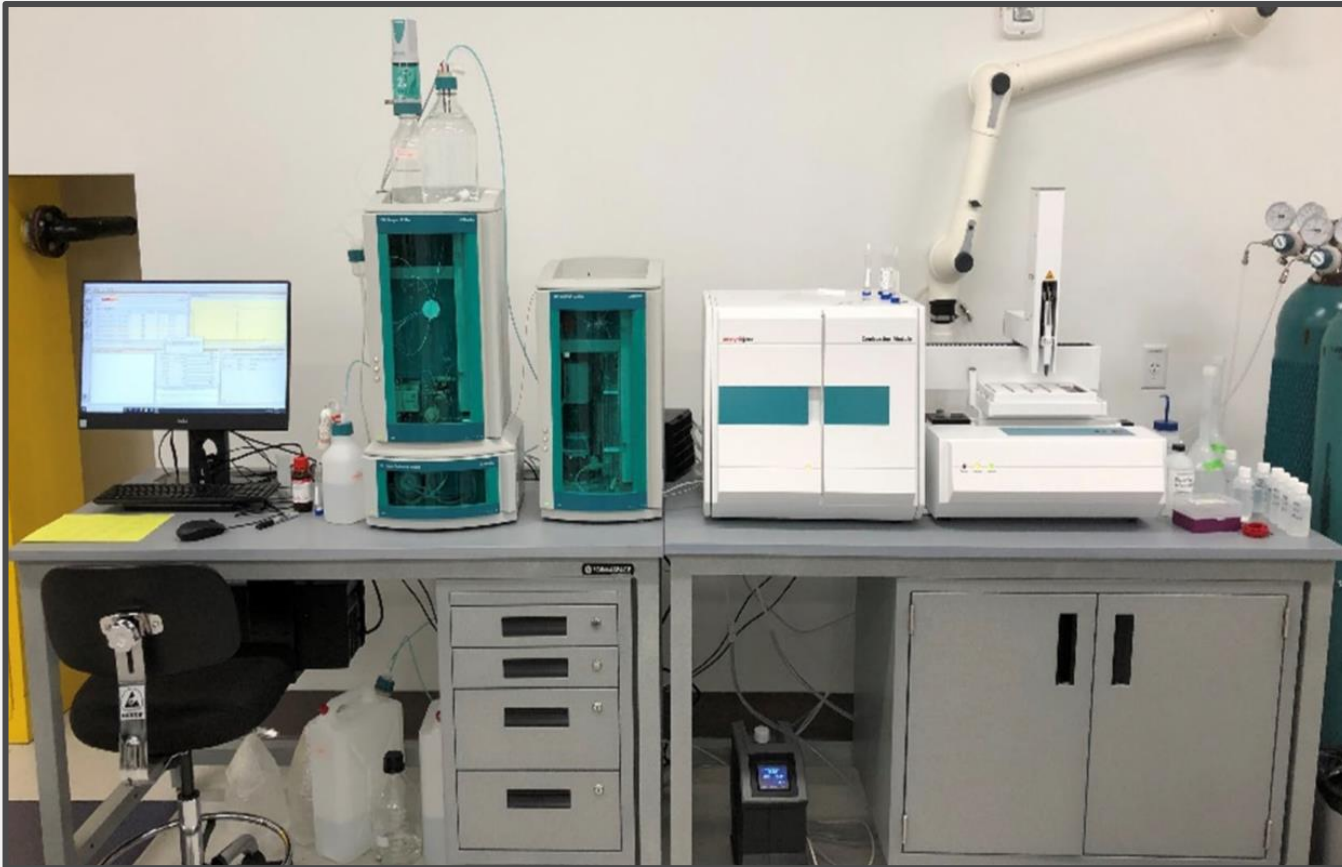
Solids Sample Configuration (AOF/EOF)
