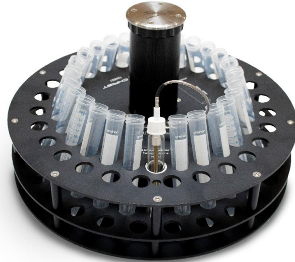
Rack for parallel processing of 23 x 15 mL Falcon™ Tubes
