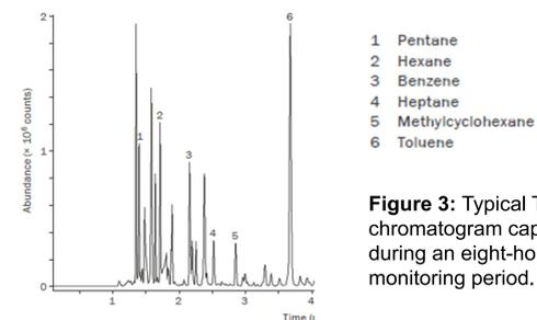
Figure 3: Typical TD chromatogram captured during an eight-hour monitoring period.
