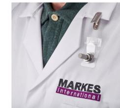
Figure 5: Markes International's radial diffusive sampler and holder, for personal exposure monitoring.
