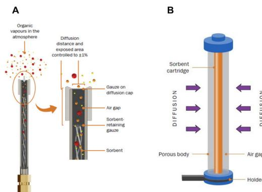
Figure 2: The diffusion process for passive samplers: (A) axial and (B) radial.
