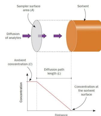
Figure 1: The principle of passive sampling.
