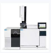
7000 and 7010 QQQ systems over 800 times more sensitive than a 5973 single quad, viable option to replace magnetic sector mass specs for dioxin/furan methodologies, GC/MS/MS allowed in the newest revision of 8270
