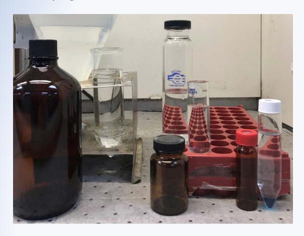
1000 mL of sample process uses approximately 200 mL of methylene chloride
