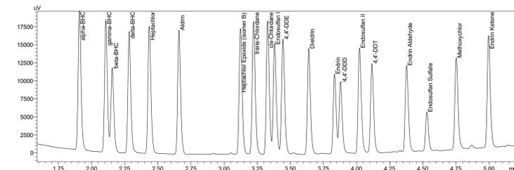
Figure 5: Chromatogram of 4 ppb organochlorine pesticides standard in hexane analyzed on Rtx-CLP column using He carrier gas.
