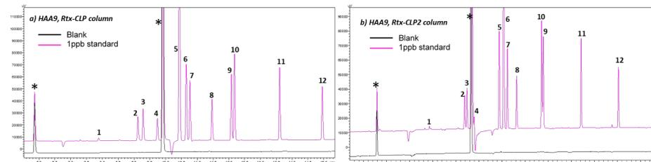
Figure 3: Chromatograms of MTBE blanks and 1 ppb HAA Methyl Ester Mix on a) analytical column (Rtx-CLP) and b) confirmation column (Rtx-CLP2) using H<sub>2</sub> carrier gas. Peaks indicated with an asterisk do not correspond to any of target peaks.
