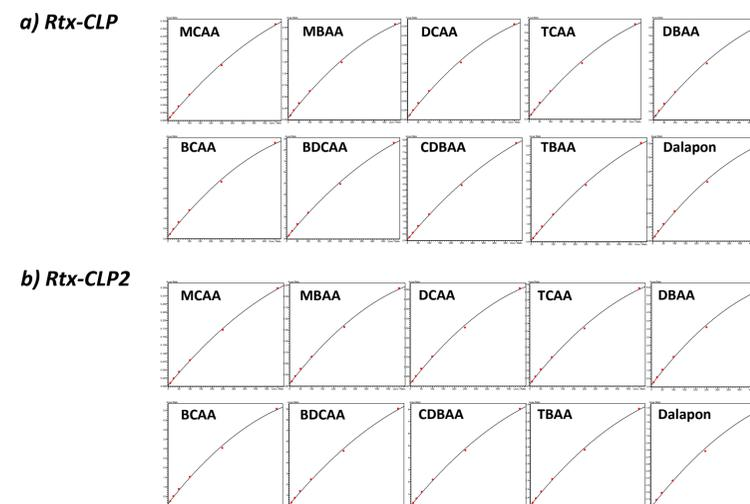
Figure 4: Six-point calibration curves for HAA9 and dalapon on a) analytical column (RtxCLP) and b) confirmation column (Rtx-CLP2) using H<sub>2</sub> carrier gas.
