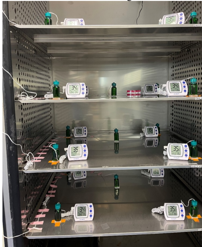
Figure 1. Example of Temperature Mapping Using Thermocouples
