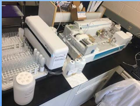
OI Analytical FS3700 Segmented Flow Analyzer,
