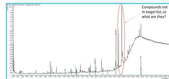
Figure 3. TIC of primary effluent sample. Compounds identified from target library have green traces with RTs. Two, high intensity peaks without green traces, indicating the compounds are still unknown are circled.
