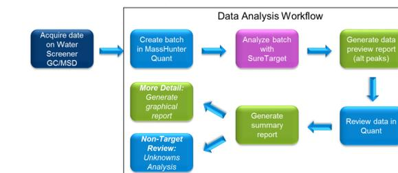
Figure 6. Suggested Data acquisition to data analysis workflow
