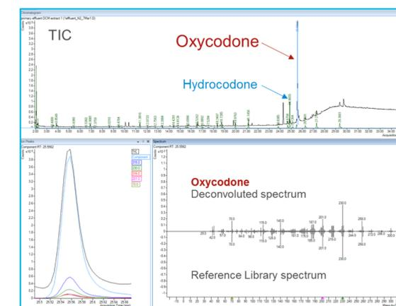
Figure 5. Unknowns Analysis screen shot with oxycodone selected in the TIC. the overlaid component, EICs, and head-to-tail comparison of the deconvoluted spectrum with NIST14 library spectrum.
