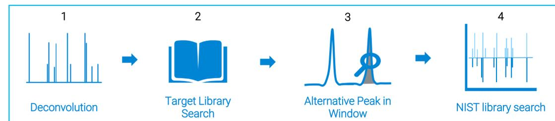
Figure 1. The four automated steps of the SureTarget workflow in MassHunter Quantitative Analysis B.08.
