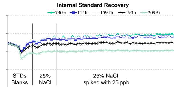
FIGURE 3. Internal std recovery during analysis of 25% NaCl samples (t=4 hrs)
