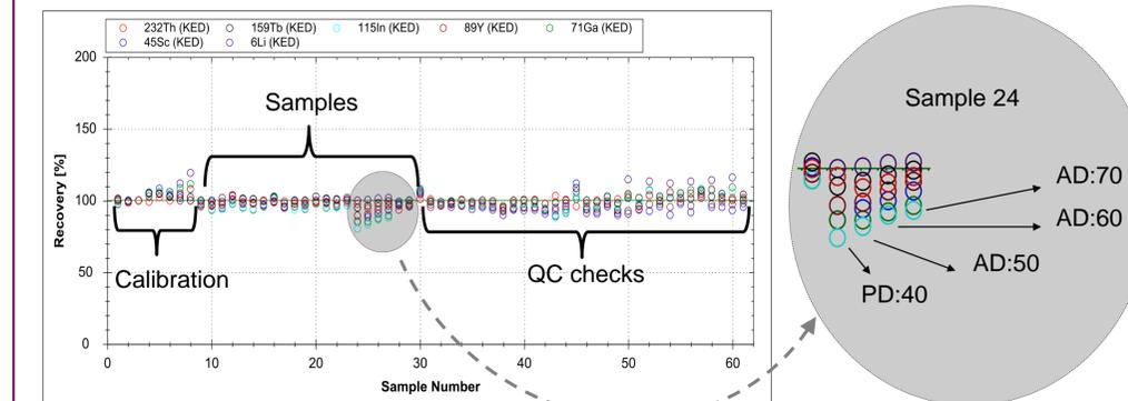
FIGURE 5. Internal standard response during semi-saline water analysis. Expanded software screenshot (right) illustrates automatic auto-dilution, triggered after analysis of Sample 24.
