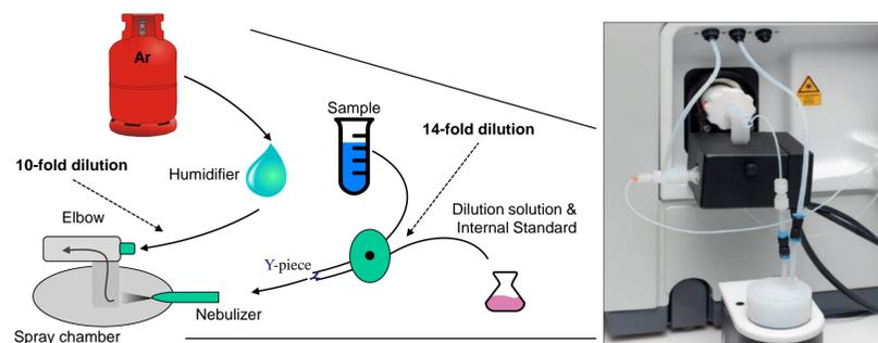
FIGURE 1 . Concept of an argon gas dilution approach coupled to online dilution.
