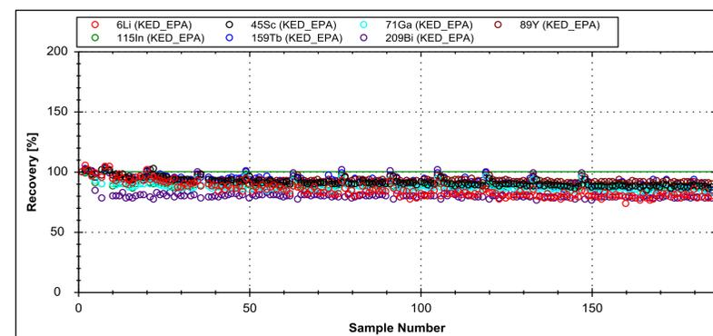
FIGURE 4. Internal standard recovery during analysis of tap water and QC samples. All recovery results are within the 60 – 125% range specified in EPA Method 200.8.
