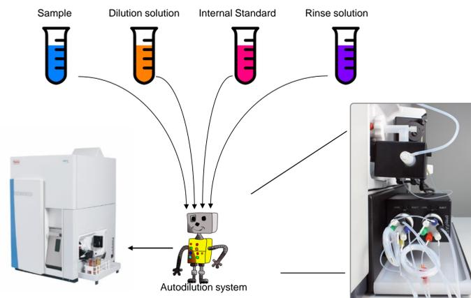
FIGURE 2. Concept of a fully automated dilution system.
